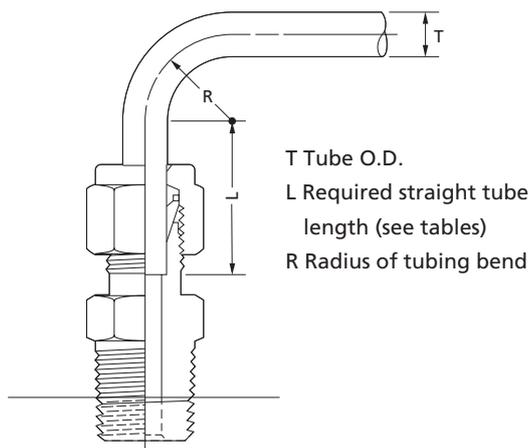
Tubing properly selected and handled, combined with properly installed FITOK tube fittings, will give you a leaktight system and provide reliable service in a wide variety of applications.
